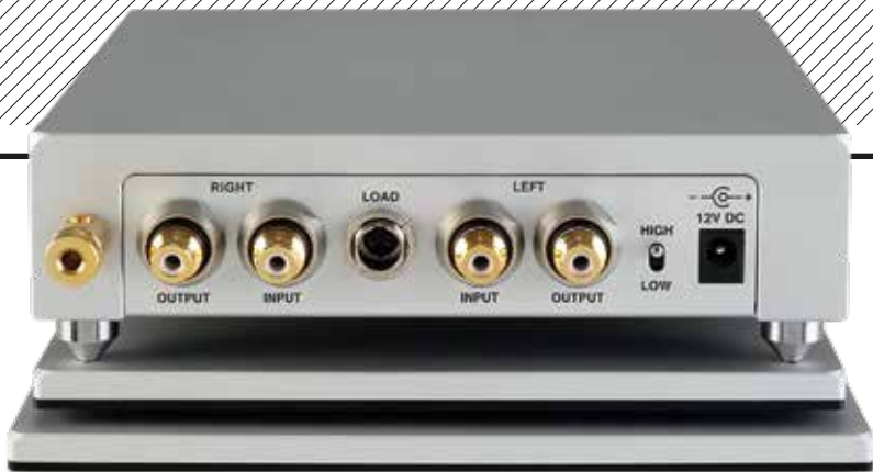
ABOVE: Single sets of unbalanced (RCA) inputs and outputs are joined by a chassis ground post, Low/High gain toggle, three-pin socket for the loading plug (default is 100ohm) and a DC input for the supplied wall-wart or optional Compact PSU
